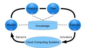
Fig. 1. Cloud computing systems with MAPE-K adaption loop.
